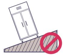
The unit must be installed on an even surface; uneven or tilted surface can make noise or/and poor performance.
