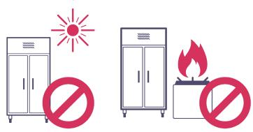
Do not place the unit in an area next to heat generating equipment or with direct sunlight.
