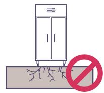
The installation surface must be capable of supporting the load of the cabinet.
